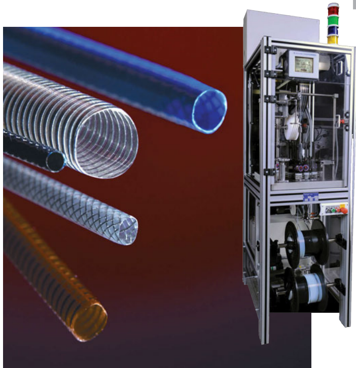
Ultra-fine wire is braided on specialized braiding equipment. Steeger machine shown above on right.
