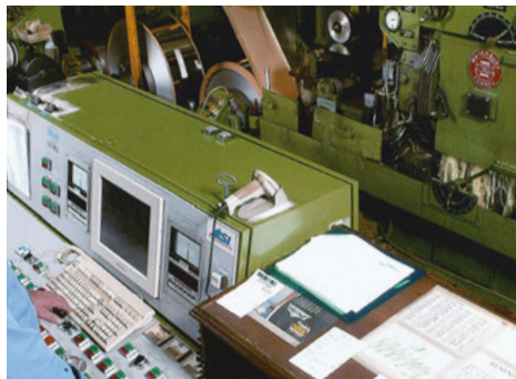
This high speed Z-mill is equipped with automatic gauge control to instantly adjust the roll bite and maintain the desired gauge and close tolerances.
