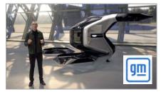
"reimagining the future of personal transportation". The single-passenger vertical take-off and landing (VTOL) drone will be able to travel from urban rooftop to urban rooftop at speeds up to 55 miles per hour. It is fully autonomous and all-electric, with a 90kW motor, a GM Ultium battery pack and an ultra-lightweight body with four pairs of rotors. (See Appendix: Automotive, page 12)
