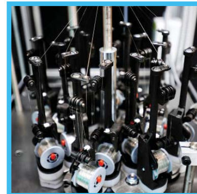
Close up of multiple bobbins wound on Steeger machine.
