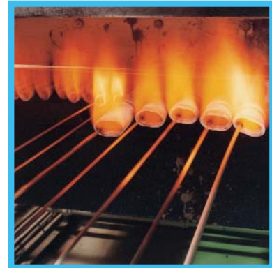
Intermediate and final strand annealing is used to control mechanical properties.
