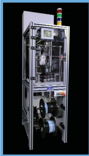
Material is wound on specialized Steeger machine.
