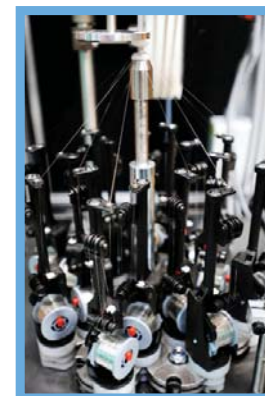
Close up of multiple bobbins wound on Steeger machine.
