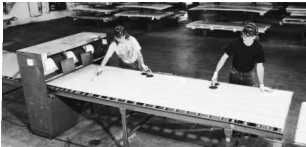
Clear or color coded coatings are applied to stainless steel sheet to protect the material during shipment and manufacture. Plastic sheeting in various mil thicknesses and levels of adhesion are available.
