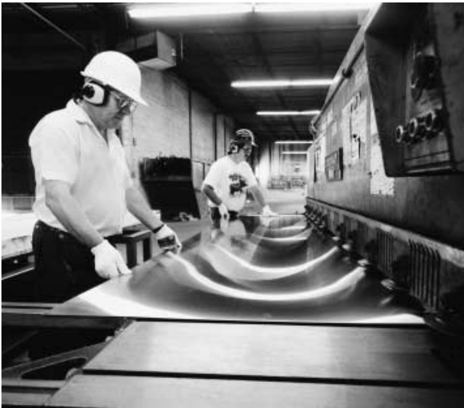
Sheet is cut to accurate lengths and widths on this high capacity shear.
